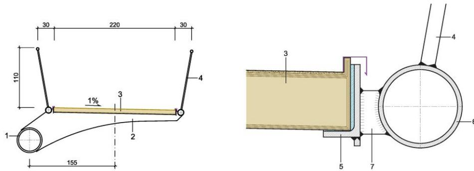
Fig. 3 a) Footbridge cross section; b) Railing connection and deck lateral flange detail, with: 1. Main beam ROR 457/40, 2. Consoles, 3. COLEVO deck, 4. Railing, 5. Lateral LNP profiles, 6. Lateral ROR 114/7 profile, 7. Spacers
