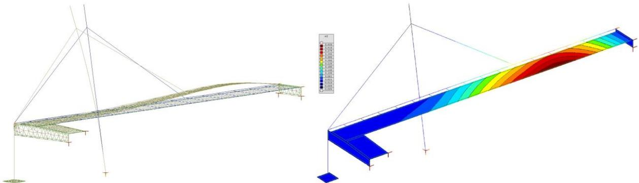
*Fig. 5 a) Eigen mode for vertical vibrations calculated using a 3D shell model (Software Axis VM,  $f = 4.56\text{Hz}$ ); b) vertical displacements*
