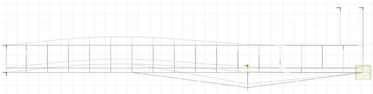
*Fig. 6 Eigen mode for transverse horizontal vibrations calculated using a 3D shell model (2.81Hz without plate action)*
